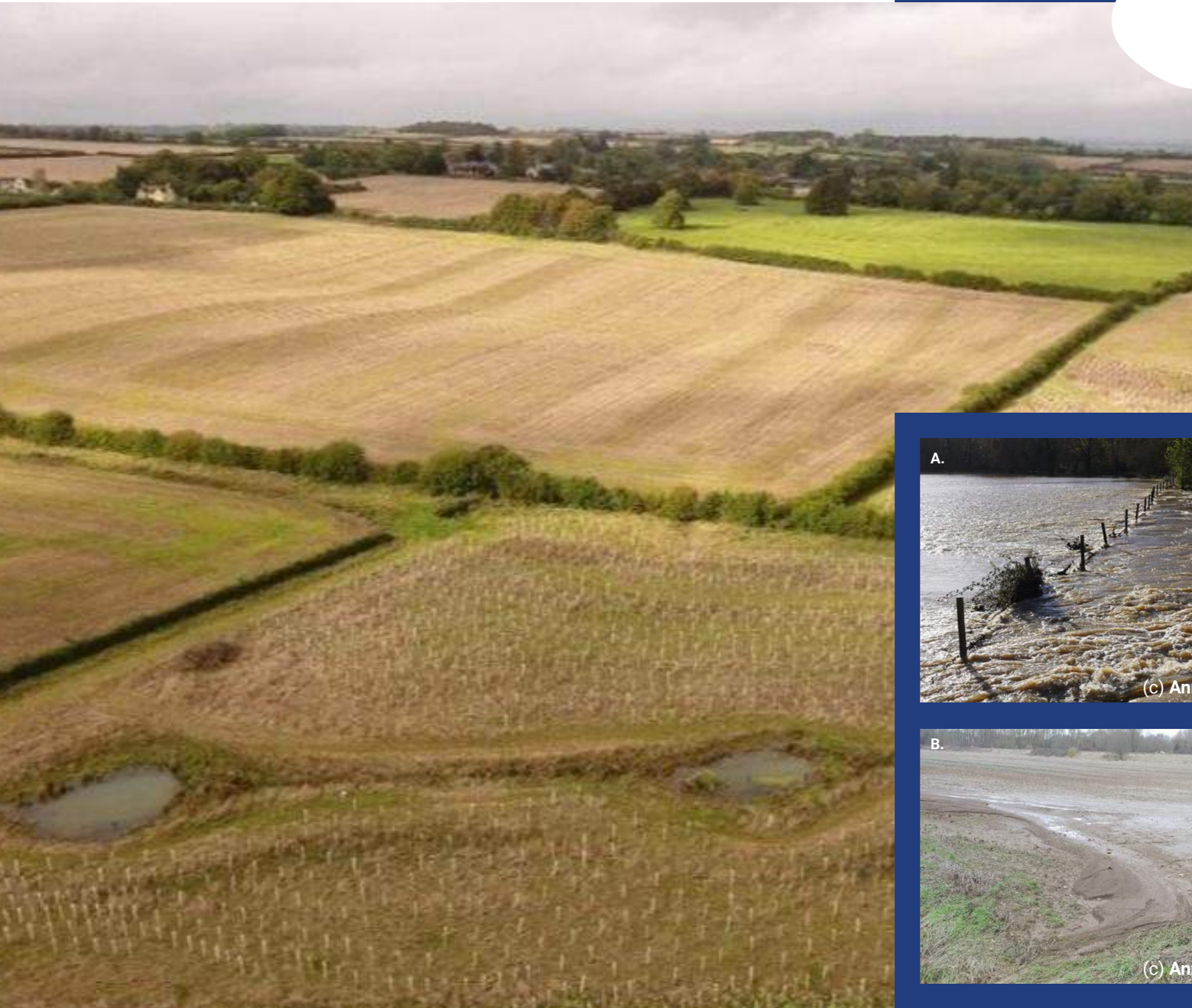
Figure 9: A series of connected ponds in the Littlestock Brook designed to capture sediment and nutrients from the surrounding farmland. (Photo: D. Gasca-Tucker).
