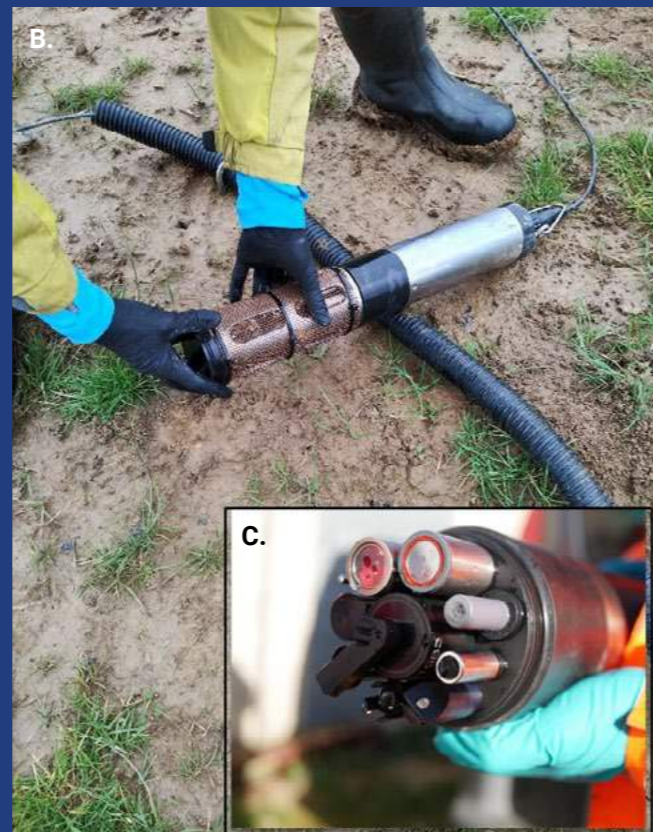
Figure 16: Maintaining a Proteus Instruments multi-parameter sonde (Photo: L. Bannatyne) INSET: Proteus sonde with the protective cage removed.
