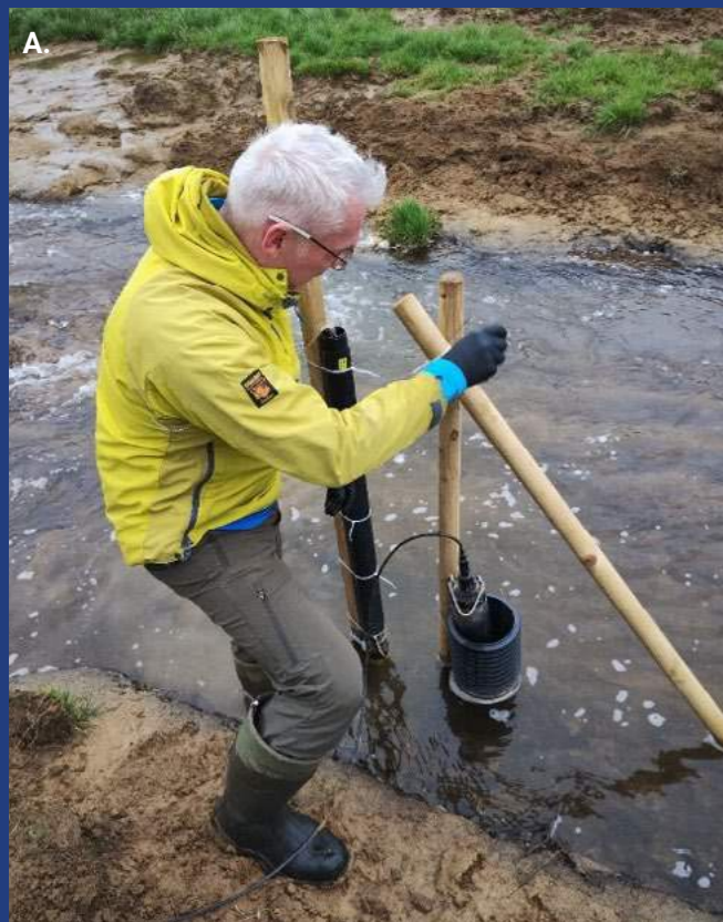
Figure 15: Near-continuous water quality monitoring. A) the proteus sonde; B) the pressure logger stilling well; C) the sonde stilling well.
